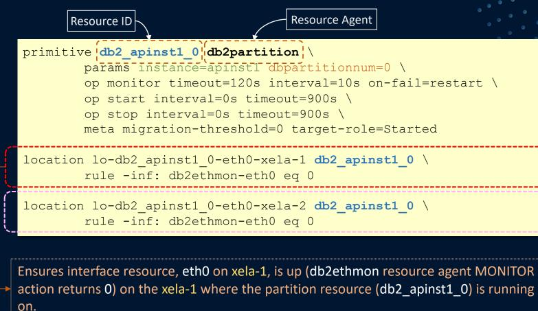
Ensures interface resource, eth0 on xela-2, is up (db2ethmon resource agent MONITOR action returns 0) on the xela-2 where the partition resource (db2\_apinst1\_0) is running on.
